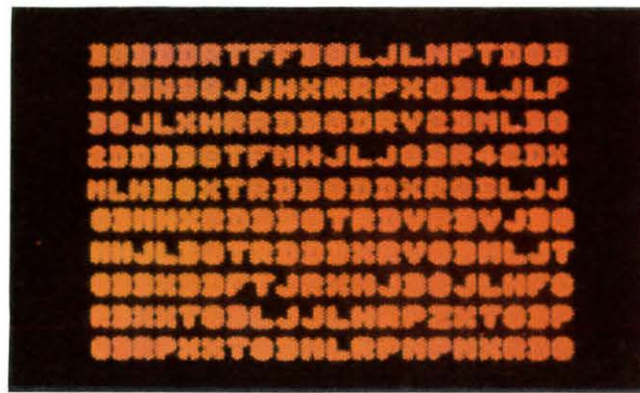
Figure 6. Photo—Alphanumeric Pattern of Entertainment 14V CRT, 3000 Characters/Frame.
